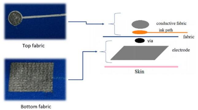
Figure 1. Sandwich structure for collection of EMG signal
