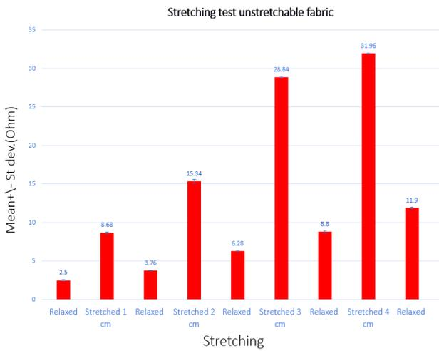
Figure 6. Stretching test results for unstretchable fabric
