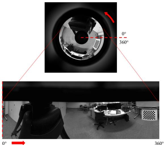
Figure 3. Example expansion of omnidirectional camera image.
