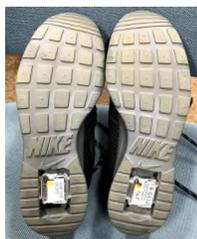
Figure 6. Sensor devices embedded into shoes.
