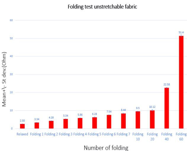
Figure 8. Folding test results for unstretchable fabric
