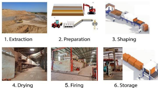
Figure 1. Manufacturing Process of SNG.
