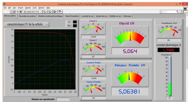
Figure 7. Dashboard of the PV system
