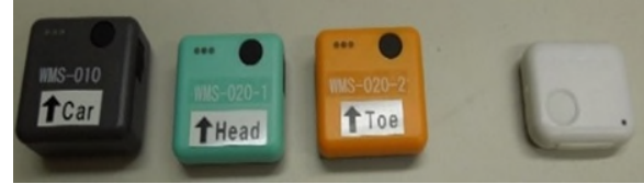
Figure 1. Wireless wearable motion sensors.
