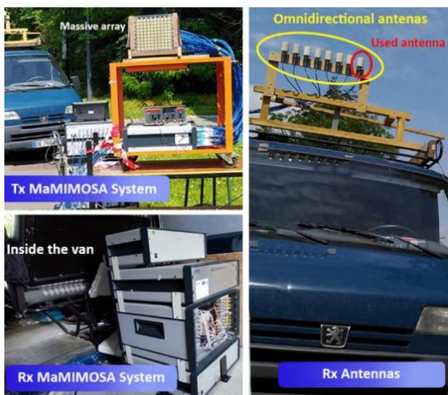
Figure 2. Tx-Rx antenna systems.
