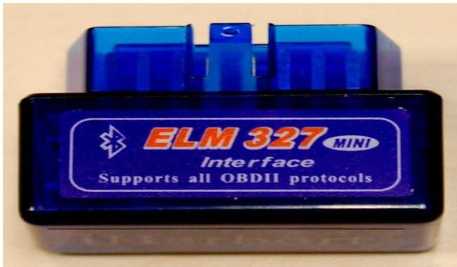
Figure 4: ELM 327 OBDII device
