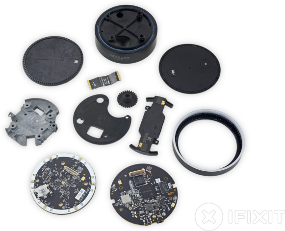
Figure 6. Teardown of the Echo Dot [5]
