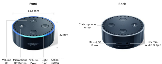
Figure 5. Basic structure of the Amazon Echo Dot [30]
