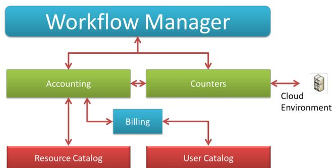
Figure 3. Communication between billing-related components inside infrastructure.
