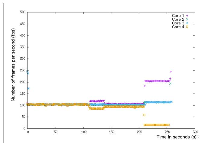
Figure 1. Memory bandwidth reservation on different cores
