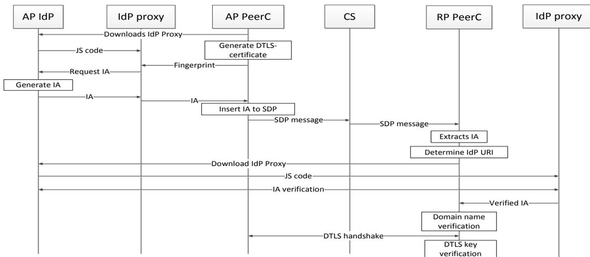
Fig. 2. End-to-End Authentication Flow Diagram
