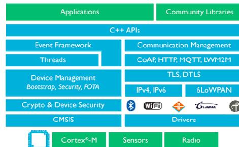
Figure 3. MBED stack from the ARM company
