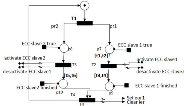
Figure 5. GR-TNCES model of an  $ECC_{controller}$ .
