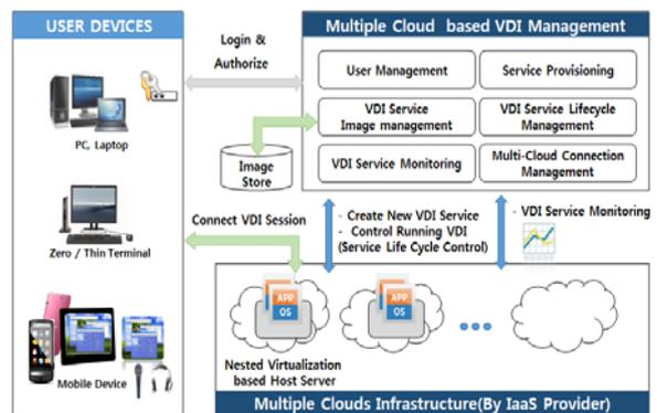
Figure 2. Architecture for multiple Clouds based VDI service
