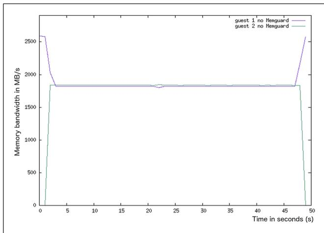
Figure 7. Memory bandwidth degradation between two guests
