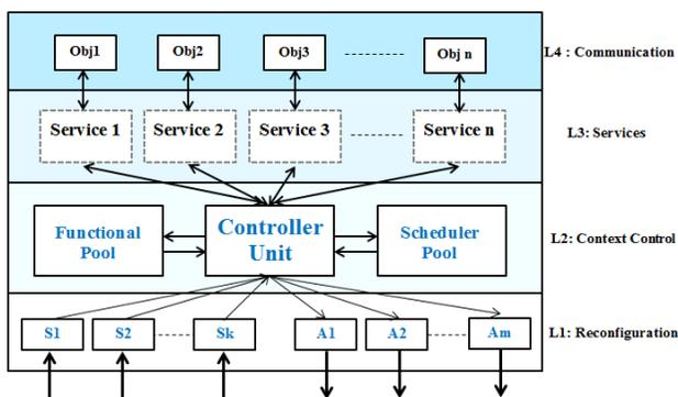
Figure 1. The modules of R2TCA layers.
