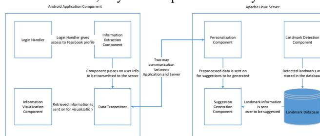
Figure 1. A diagram of the proposed system.
