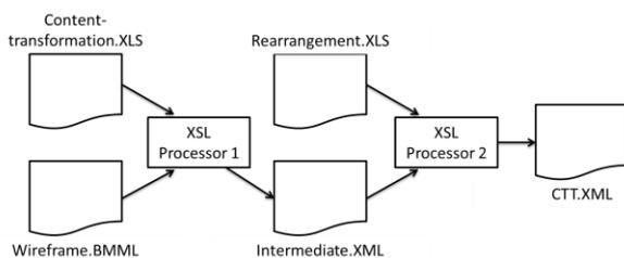
Fig. 1. Illustration of the two-step transformation from Balsamiq's specific BMML file format into the UI model in CTT notation.
