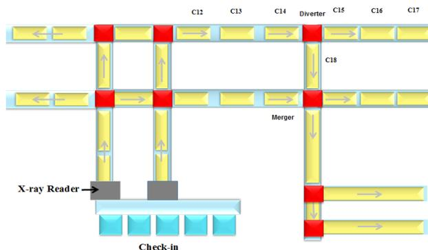
Figure 8. The baggage handling system structure.
