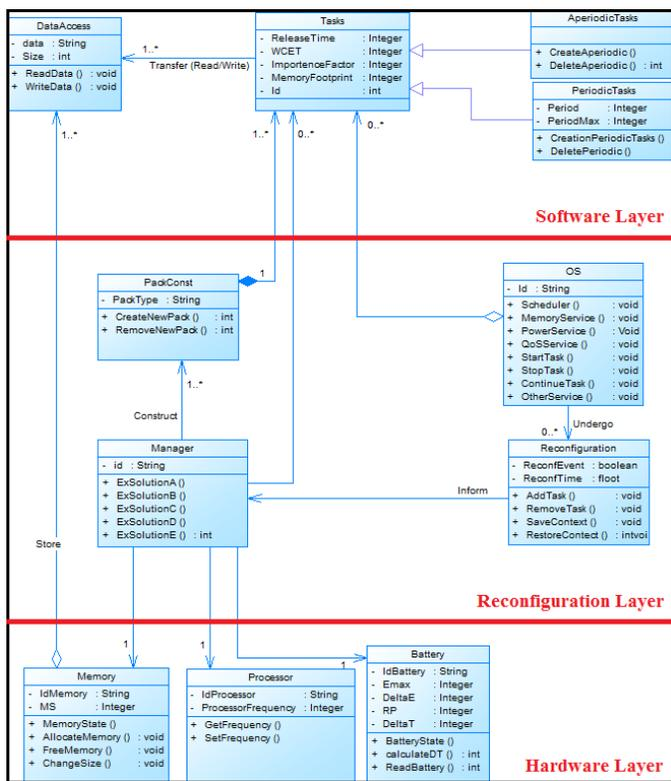
Figure 4. Class Diagram.
