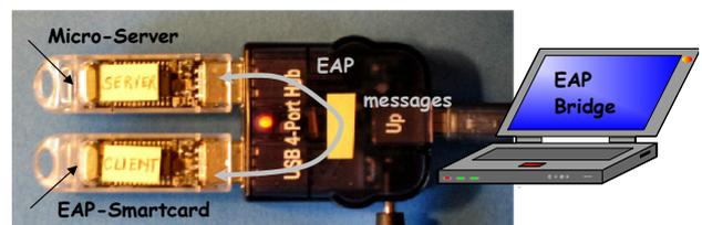
Figure 4. The first TLS micro-authentication server [15], 2005
