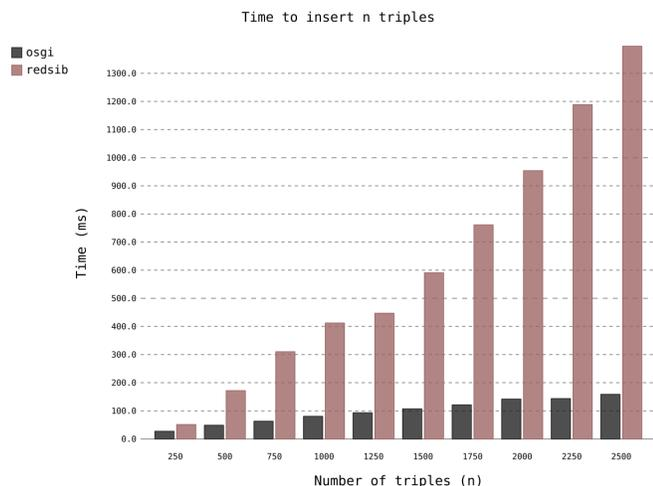
Fig. 3. The Update test performed on RedSIB and OSGi SIB
