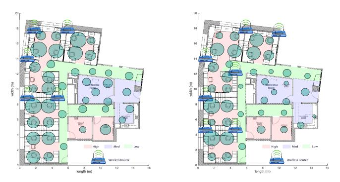
Figure 7. Visualization of IPS configuration in CREST for experiment A (left) and B (right), where 5 or 7 access points are deployed according to APEC Greedy. Location priority map is color coded as illustrated in the legend. Location frequency map is not shown, which is HIGH for cubicles, MED for shared spaces, and LOW for corridors. The radius of the green circle indicates the number of fingerprints at the spot.
