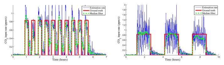
Figure 10. Sensing the latent CO<sub>2</sub> emission rate by proxy for CO<sub>2</sub> pump experiment A (left) and experiment C (right). The estimated emission rate (blue), median filtered rate (green), and ground truth (red) are given.
