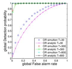
Figure 5. The ROC curves of the OR fusion
