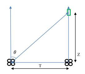
Figure 7. Classical stereo vision method for the stationary pedestrian
