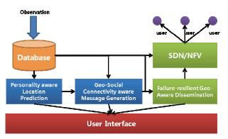
Figure 2. The architecture of the proposed disaster warnding system
