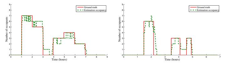
Figure 11. Occupancy detection by "sensing by proxy" (Algorithm 1) for experiment E (left) and G (right). The response times from vacancy to occupancy and vice versa are about 10 seconds and 5 to 10 minutes respectively, since the method detects the dynamics of the system rather than static concentration. The estimations (green) are within 1 occupant of the ground truth (red).
