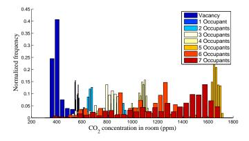
Figure 6. Empirical distribution of CO<sub>2</sub> concentration for all occupants experiments corresponding to different occupancy (color coded).
