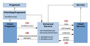
Figure 5. Universal service handles binding of client services.
