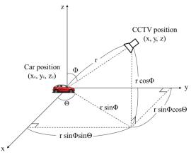
Figure 15. Construction of arbitrary views
