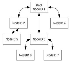
Figure 1. A typical RPL DODAG with one root and six other nodes.
