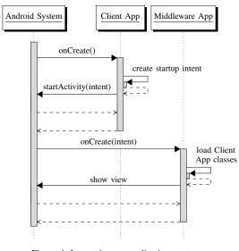
Figure 4. Interaction on application startup.
