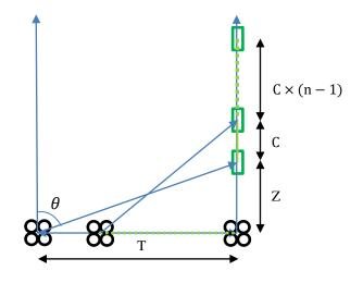
Figure 9. Geometry for pedestrian moving perpendicular to the baseline
