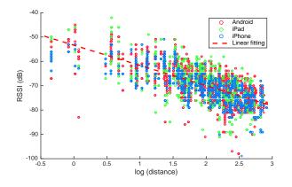
Figure 4. Plots of RSSI vs. log distance color coded by devices. A linear regression line is fitted on the data:  $RSSI = -8.31 \cdot \log(d) - 53.4$ .
