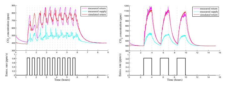
Figure 7. Proxy model simulation with CO<sub>2</sub> pump experiment A with 30 minutes (left) and experiment B with 1 hour (right) periodic excitation. Measurements at supply (green), return (blue), and simulated return (red) vents are shown.
