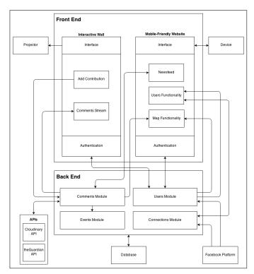
Figure 1. High-Level Block Diagram of the system
