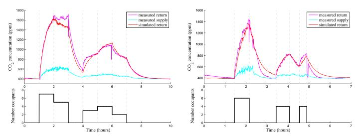
Figure 8. Proxy link model simulation with occupants experiment E (left) and G (right). The proxy measurements at return (blue), supply (green), and simulated return (red) vents are demonstrated.
