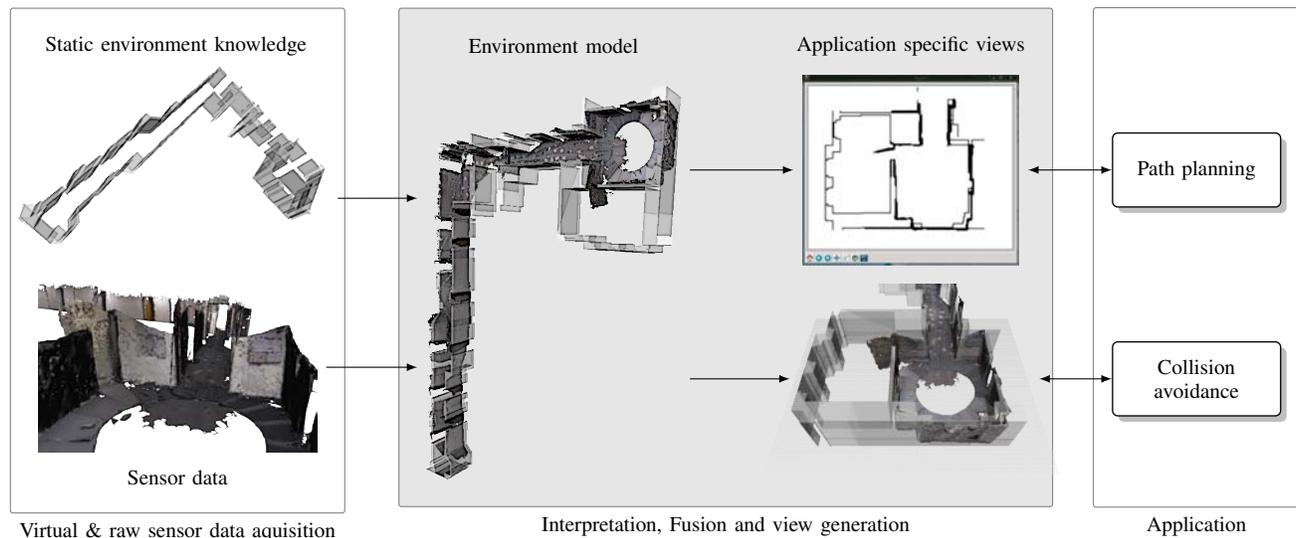
Fig. 3: Composing an environment representation from static & dynamic data and generate of application specific views from it.
