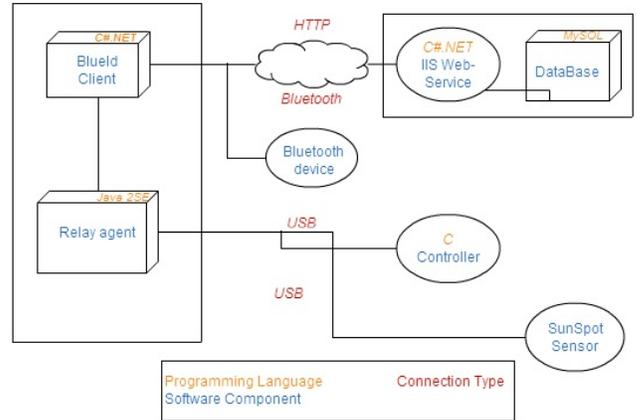
Fig. 2. System's Architecture
