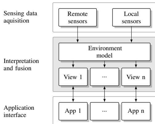
Fig. 2: View generation related to application requirements and based on a common environment representation.
