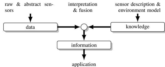
Fig. 1: Relation between sensor data and application specific information.
