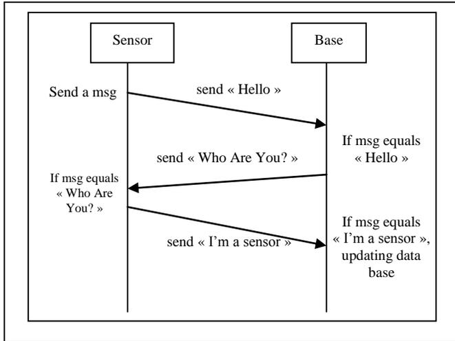
Figure 3. Communication protocol based on soft security
