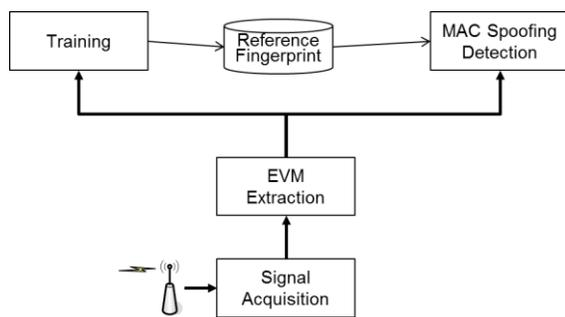
Figure 2. Architecture for MAC spoofing attack detection.
