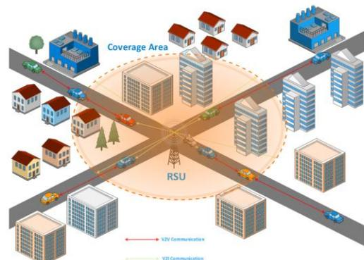
Figure 1. Communication architecture of VANET.
