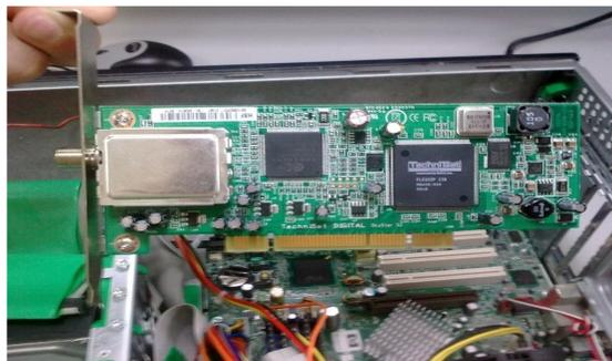
Figure 6 – Technisat™ SkyStar 2 DVB PCI Card
