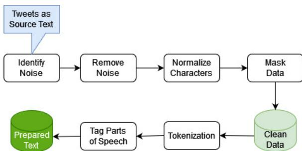
Fig. 1. Pre-Processing Pipeline
