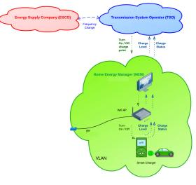
Figure 7. Testbed infrastructure
