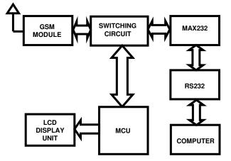
Figure 1. Block diagram of the system.
