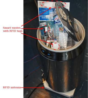
Figure 6. An individual bin using the RFID technology.
