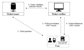
Figure 3. Architecture of the identification-based model
