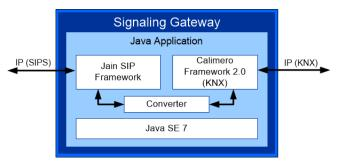
Figure 3. Connection interfaces of the Signaling Gateway
