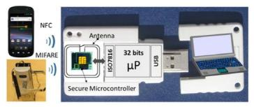
Figure 2. Triple Interface Secure Token (TIST) hardware architecture
