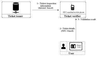
Figure 5. Architecture of the smart card-based model
