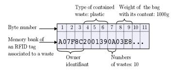
Figure 9. Data memory structuration of a smart trash bag.
