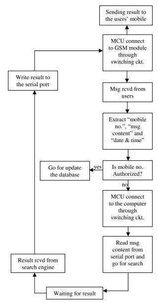
Figure 2. MCU functional diagram
