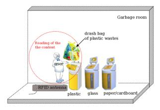
Figure 11. An individual bin using the RFID technology.
