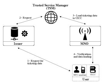
Figure 1. Architecture of the operator-centric model
