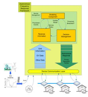
Figure 6. Autonomous frequency response framework
