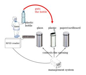
Figure 5. A RFID based selective bin.
