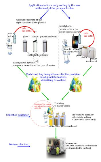
Figure 1. Waste flow and global architecture of the system.
