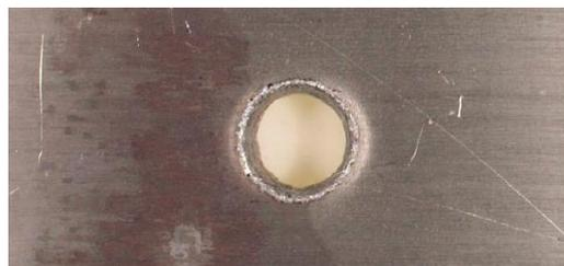
Figure 6. Front view of a perforated aluminum 0.5 inch thick target.
