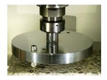
Figure 3. Scratch Test Device on Basalt.
