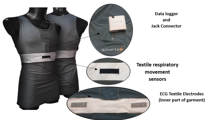
Fig. 1. Wearable sensing platform architecture.
