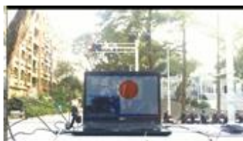
Figure 6. Daytime traffic light captured and recognized.
