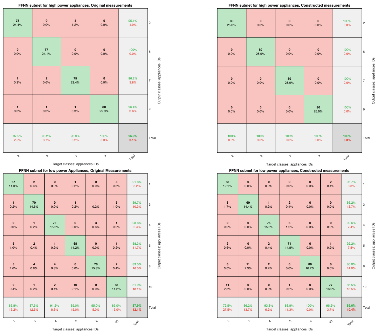
Figure 7. Confusion matrices for FFNN classification results on original measurements (left), and constructed measurements (right)
