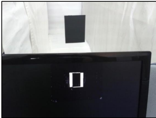
Figure 5. The disparity map for a zero disparity level at 1 meter distance. from the cameras
