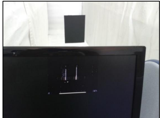
Figure 8. Disparity map for (0010111)_2=(23)_{10} disparity level at one meter from the cameras
