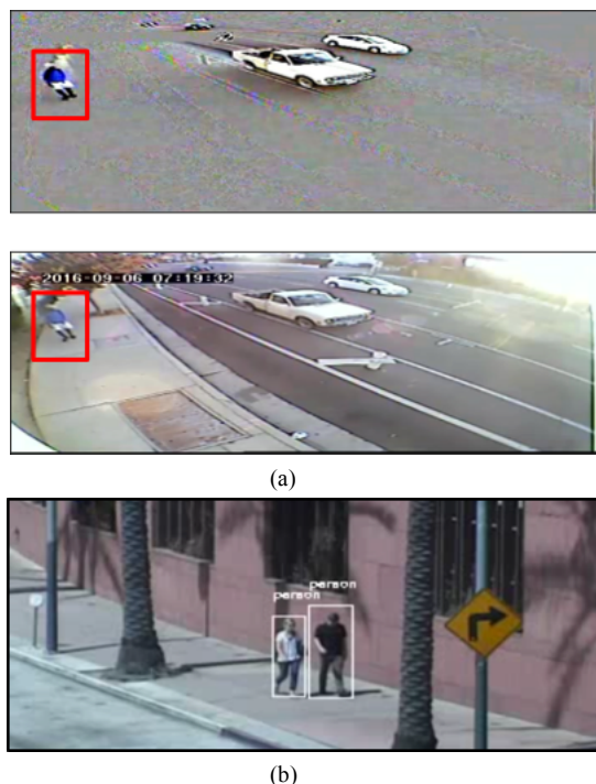
Figure 5. Pedestrian detection using machine learning algorithms. (a) using HOG features and SVM classifier, (b) using YOLO.
