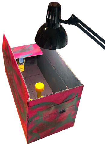
Figure 1. General schematic of the experiment, showing the dark chamber with the LED lamp, a conceptual robot model, and the lux meter.
