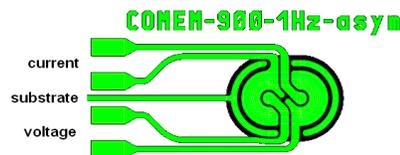
Figure 3. Typical sensor layout for four-wire measurement
