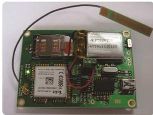
Figure 3. Photo of the “based device” to receive SMS data and subsequent visualization of the results on the map.
