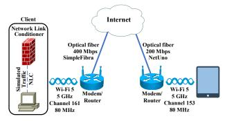
Figure 1. Testbed for Measurements
