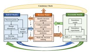
Figure 3 . An example for iterative architecture modeling process that integrates DoDAF models, executable models, and decision models.
