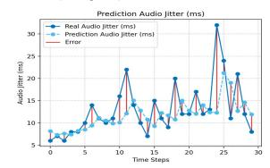
Figure 11. Actual Test Data vs. Model Prediction for Audio Jitter in Last-Minute Scenario 2
