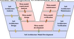
Figure 6 . SoS architecture design process with meta-model development.
