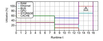
Figure 5. I/O Component Utilization after Simulation without Optimization.
