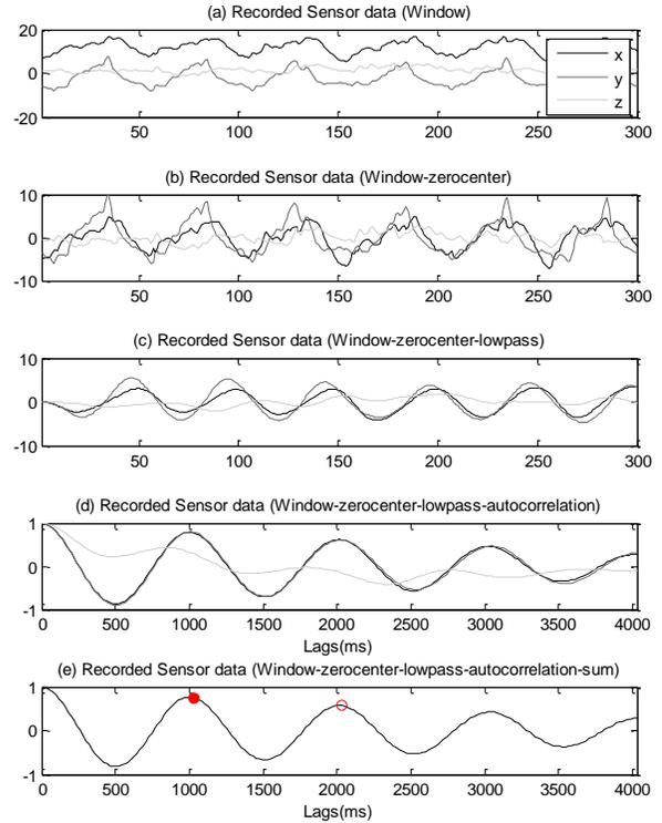
Figure 3. Recognizing pace from acceleration sensor data
