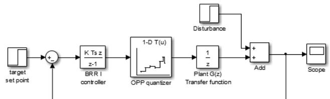
Figure 4. Diagram of the system simulator with disturbance input.
