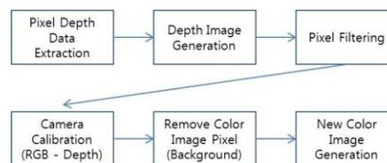
Figure 1. Pipeline of the 2-Layer Composition Module
