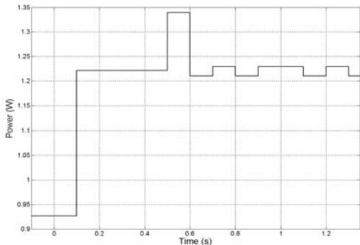
Figure 6. Closed-loop time reponse for an OPP1 to OPP15 input step and disturbance of 40% at  $t=0.5s$ .
