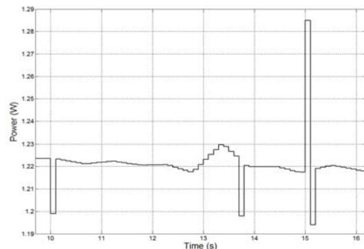
Figure 7. Closed-loop reponse for OPP15 target and noise disturbance.
