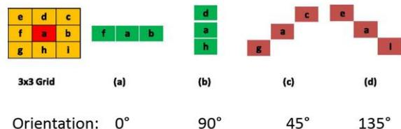
Figure 1. 3-element vector extraction [11]
