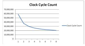
Figure 7. Perfomance Test (clock cycles / no of cores).
