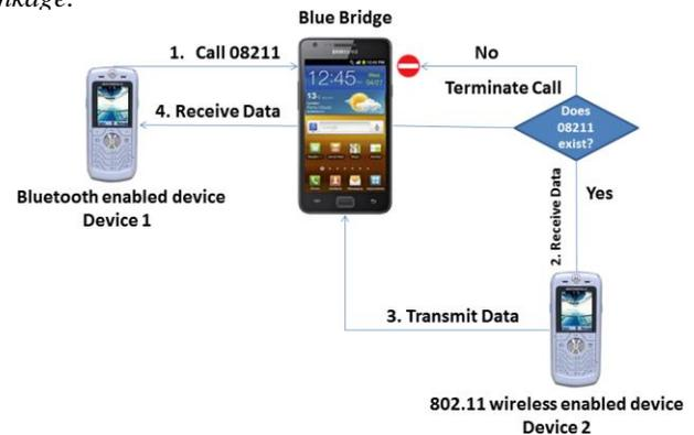
Figure 3. Linkage controlling a call between two phones
