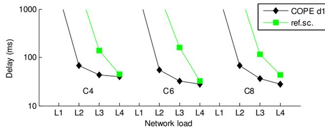
Figure 5. QoS of Case 1 - End-to-End delay for different loads in all of the observed topologies for nodes using COPE and for reference without COPE.
