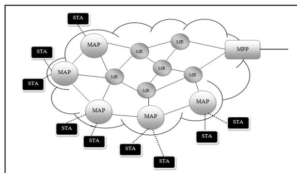
Figure 1. Network architecture of Wireless Mesh Network
