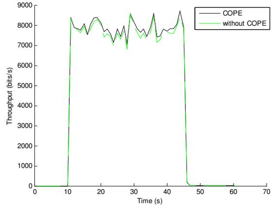
Figure 4. Network throughput for C6, L3, in case of using COPE and without COPE.
