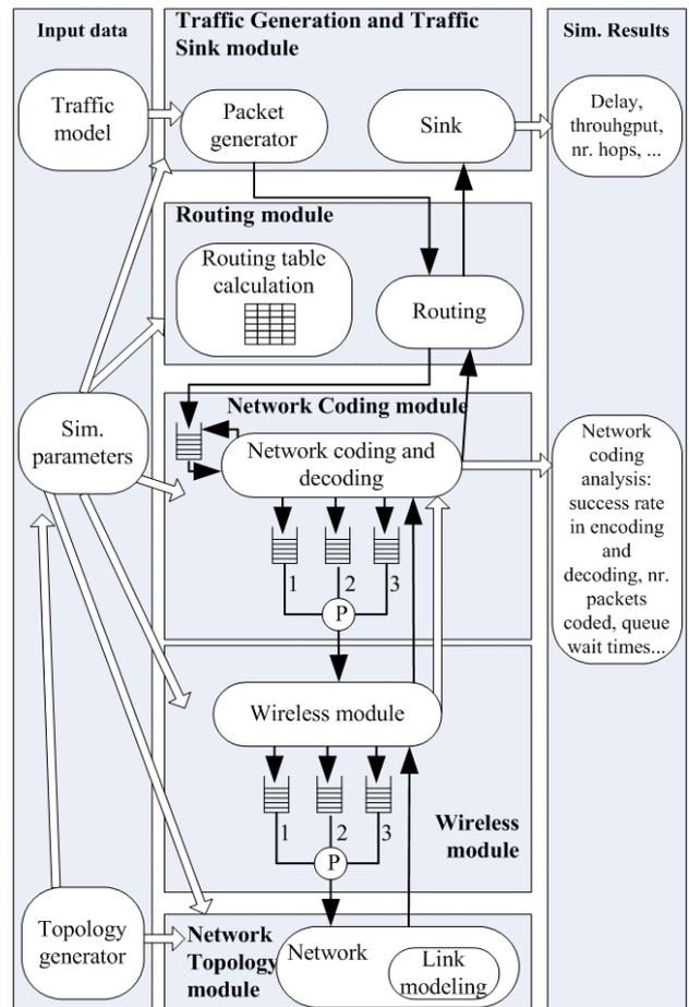
Figure 1. Network coding simulation model architecture.
