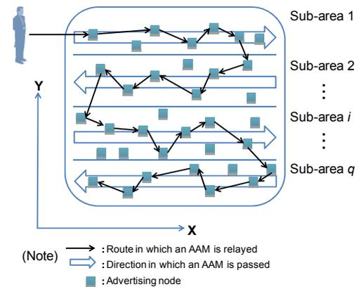
Figure 5. Example of the relay routing based on area division.
