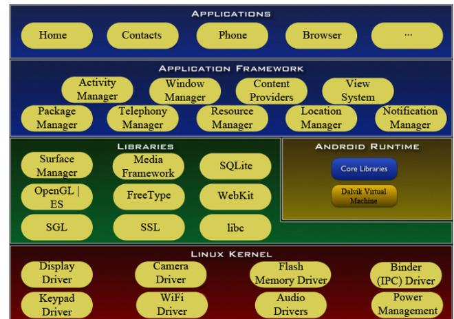
Figure 1. Android component stack
