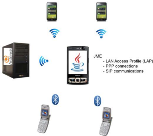
Figure 2. Proposed cell phone based infrastructure for low cost community telephone network.
