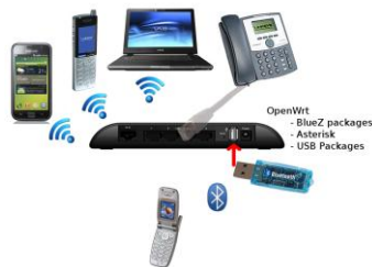
Figure 1. Proposed OpenWrt infrastructure for low cost community telephone network.
