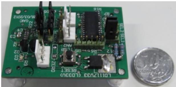
Figure 4. Intelligent Sensor Module (ISM).
