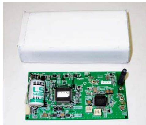
Figure 6. The case and IC motherboard developed for an EH-tag.
