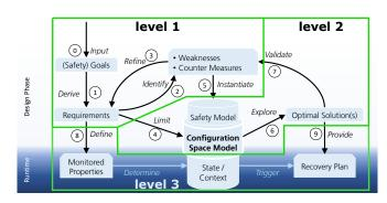
Fig. 2. Underlying structure for the iterative design and evaluation process of the dependable system architecture (detailed form)
