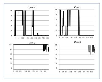
Figure 3. Per-core utilization for four-program workload broken down by core
