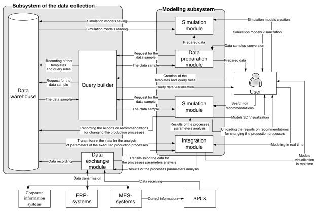
Figure 1. Architecture of the metallurgical enterprise information system
