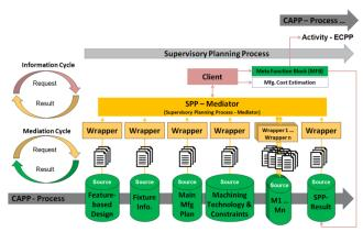
Figure 9. First level Mediator Architecture using for SPP
