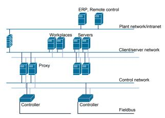
Figure 3. Traditional DCS network architecture
