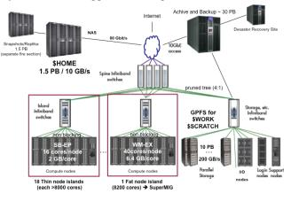
Figure 1. SuperMUC System Architecture
