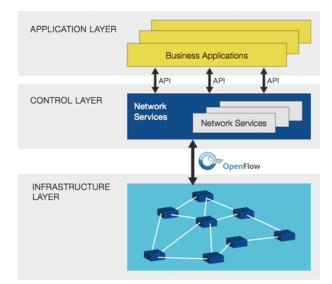
Figure 2. Three layer SDN architecture [12]
