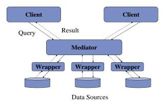
Figure 3. Mediator architecture integrating data sources
