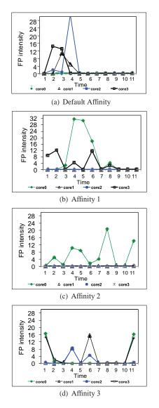
Figure 7. Variations in arithmetic intensity for different affinity configurations *wkld4*
