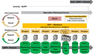
Figure 11. Third level Mediator Architecture using for OPP
