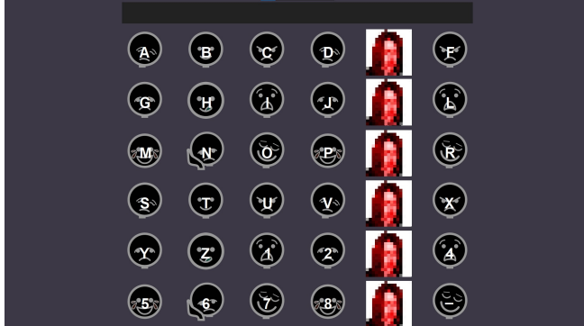
Figure 3. Interface used during the calibration task. The highlighted fifth column illustrates the stimulation mechanism of the row-column paradigm (RCP), in which entire rows and columns of the matrix are sequentially intensified. The face stimulus shown in the figure has been pixelated for copyright reasons.
