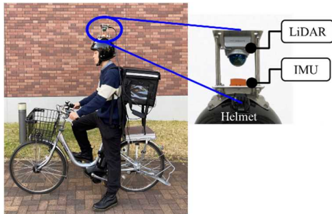
Figure 1. Overview of the experimental helmet equipped with LiDAR and IMU.
