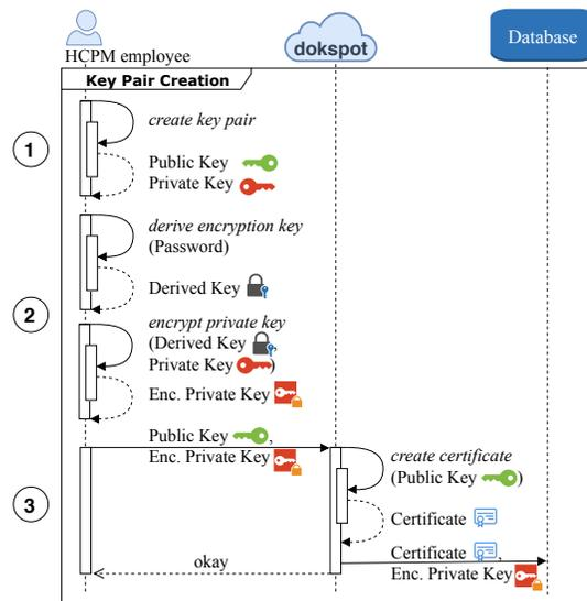
Figure 6. Key Pair Creation Sequence Diagram
