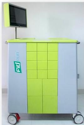
Figure 2. FIDRUN with fours modules. The first two at the top have each six small drawers and two modules at bottom have each two large drawers.
