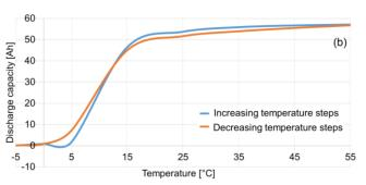
Figure 7. Battery charge and discharge capacity at rising and falling temperatures.
