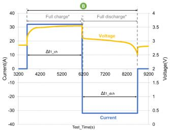
Figure 6. Calculation curve for load capacity/discharge
