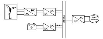
Figure 1. Electrical synoptic of the system.
