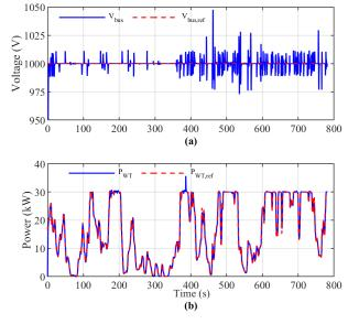
Figure 10. Comparison of measured and reference (a) DC-bus voltage (b) WT power output during control operation.
