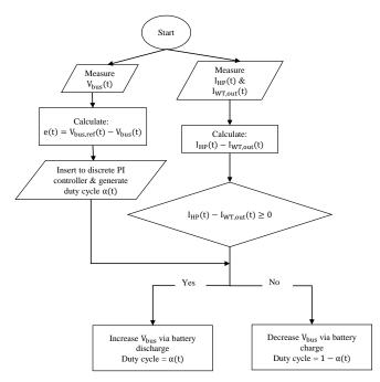
Figure 8. Buck and boost modes algorithm for the BESS bidirectional
