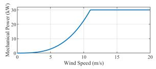
Figure 6. WT power curve.
