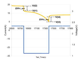
Figure 5. Voltage and current obtained during a discharge operation with a constant current of  $I_{\text{bat}} = -50A$ .
