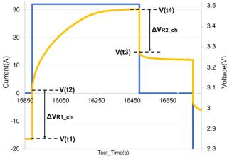
Figure 4. Voltage and current obtained during a charge operation with a constant current of  $I_{\text{bat}}$  = 50A.
