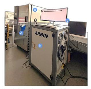
Figure 1. Test bench: (a) Computer running MITS-Pro software, (b) Battery cycler, (c) Climatic chamber (d) Battery pack.
