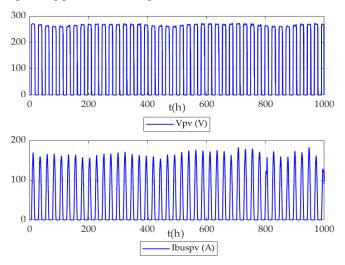
Figure 7. Waveform of the current and voltage on the PV side.
