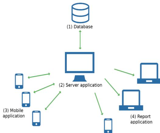
Figure 1. The client-server architecture used in the system.
