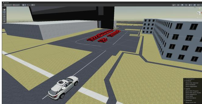
Figure 9. Lanelet2 map and 3D model imported into AWSIM.
