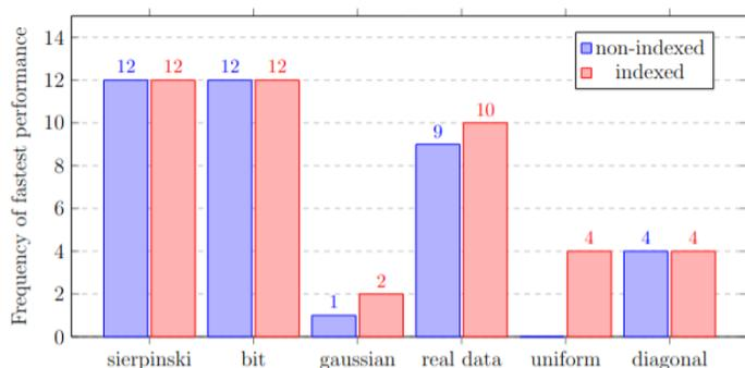
Figure 8. Frequency of DPS achieving fastest query execution across data distributions.
