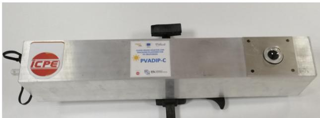
Figure 5. The physical construction of the sensor platform
