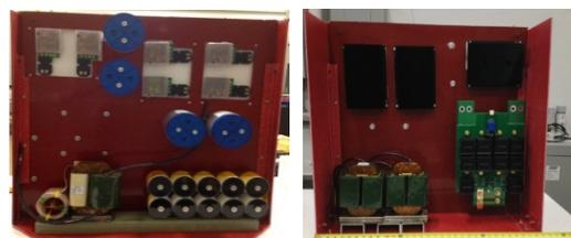
(a) Front side: High voltage side; (b) Back side: Low voltage side
