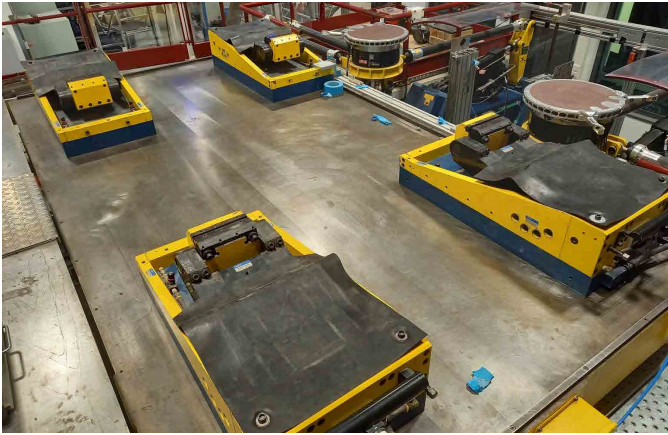
Figure 1. Main table of the test bench and its four electromagnets [43]. Four powerful electromagnets are placed on the main table, to which the car sill or a suitable adapter can be clamped.
