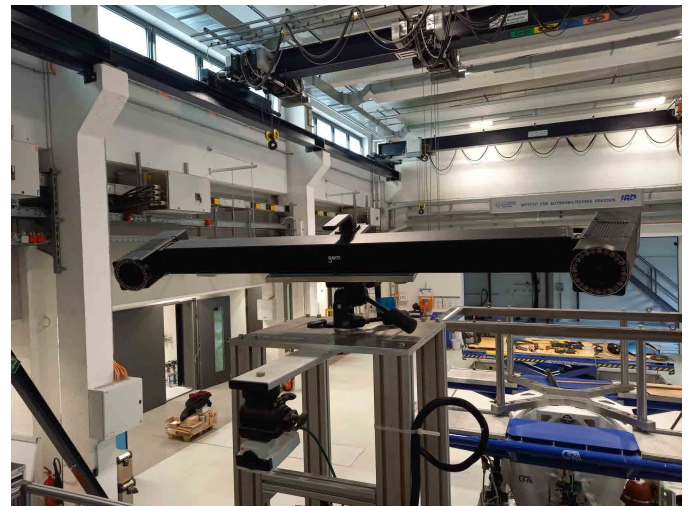
Figure 3. IT concept of the "Aramis SRX optical measuring system" test stand [43].
