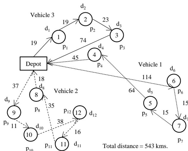
Figure 1. Graphic structure of the VRPSPD for three vehicles.
