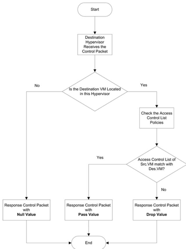
Figure 4. Destination hypervisor’s tasks after control packet reception.
