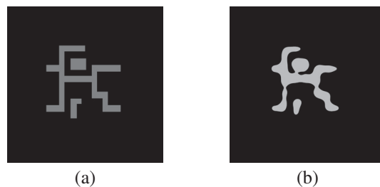
Figure 3. Hotspot: (a) mask pattern, (b) its transferred image
