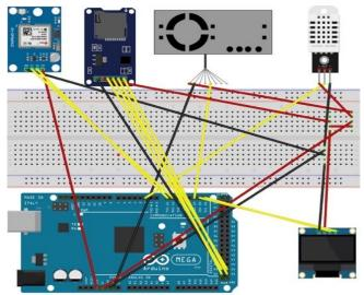
Figure 2. Schematic wiring diagram of all hardware connections.
