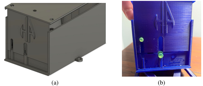
Figure 6. (a) A secondary interior wall and external overhangs overlap with attaching sections to prevent water from being introduced. (b) Opening capsule shows moisture behind slide-in wall having been stopped by the protective wall.
