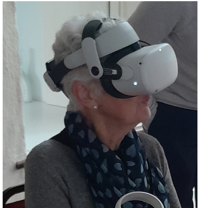
Figure 5. We replaced the original elasticated strap for the headset with a more mechanical strap that distributes the weight of the VR headset equally.
