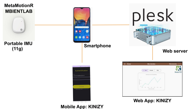
Figure 10. Axe 3 devices : MetaMotionR IMU and data acquisition architecture.
