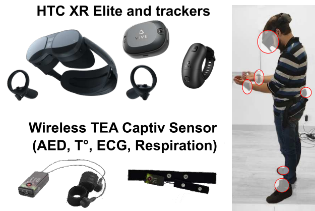
Figure 8. Axe 1 devices: HTC XR Elite and TEA wireless sensors.
