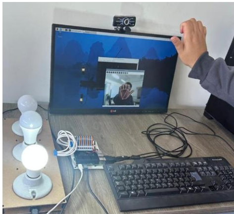
Figure 16. Gesture D, Spotlight on/off.
