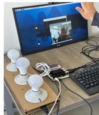
Figure 15. Gesture B grants access to the “power-on menu”.
