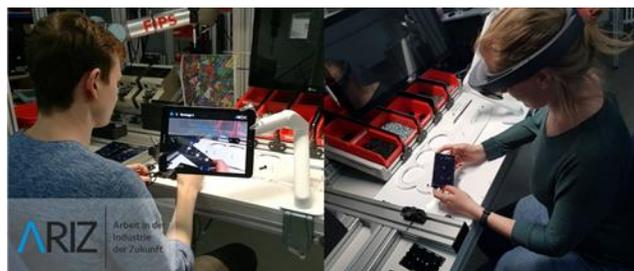
Figure 2. AR as Instructional Tool for HMD and Tablet.
