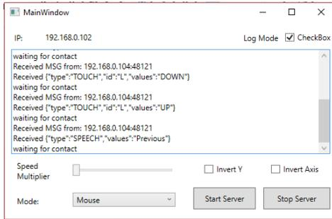
Figure 5. User Interface of the server application. The received data packets from the smartwatch are displayed for debugging purposes.
