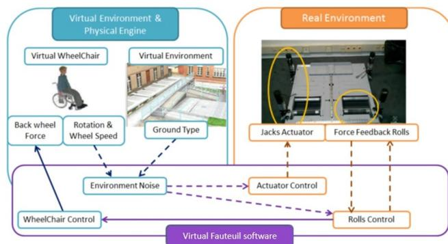
Figure 3. Communication diagram between simulator devices and the virtual environment
