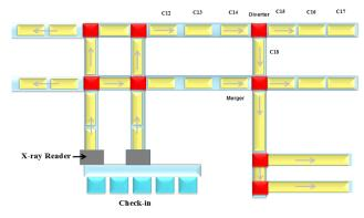
Figure 8. The baggage handling system structure.
