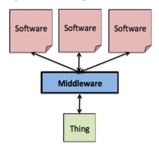
Figure 2. Interaction between software and things using middleware [12]
