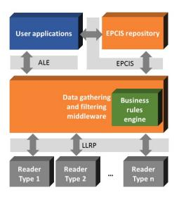
Figure 7. RFID management software architecture
