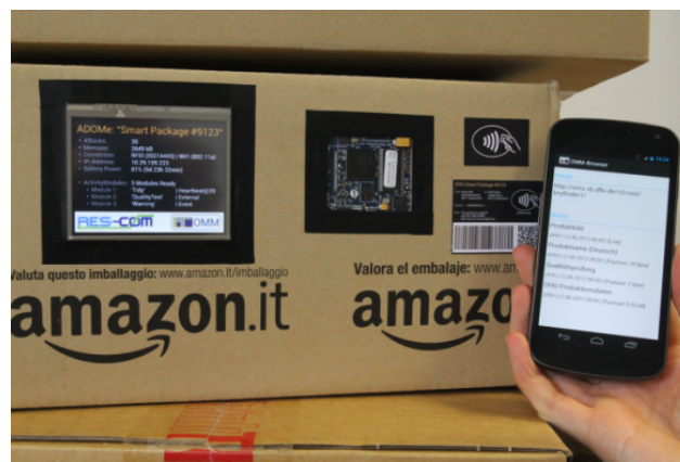
Fig. 3. Performing built-in and on-product integrity check on a smart package equipped with ADOME and accessed by a mobile handheld device.
