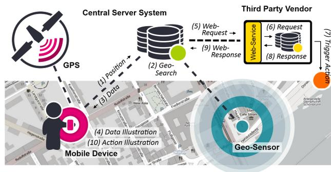
Figure 3. Geo-Sensor Architecture.
